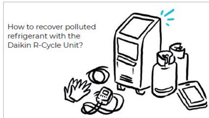
Figure 1: The basic tool components of the applied F-gas recovery process.
