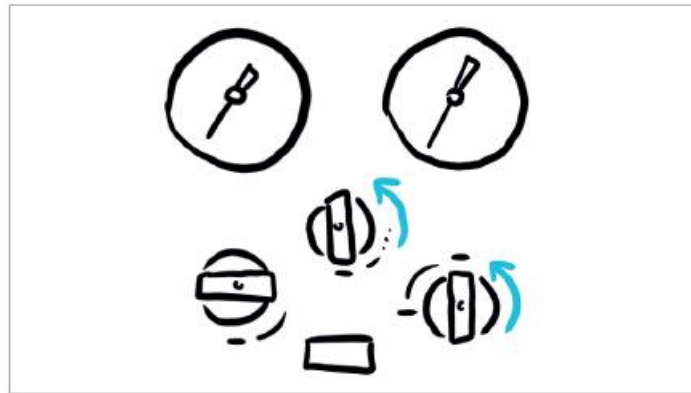
Figure 7: While the unit is off, turn the switch to purge in order to purge the remaining refrigerant from the unit. When the unit stops, close all valves. (Step 5)
