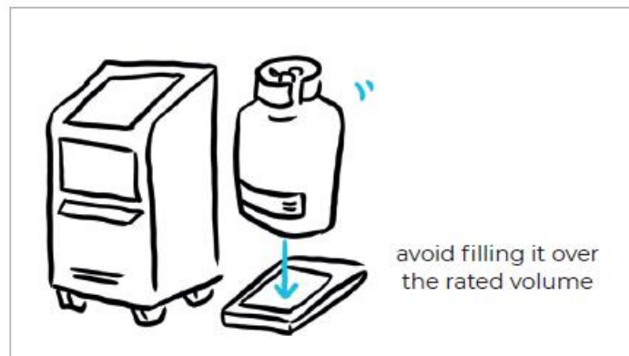
Figure 2: Place a clean and vacuumized cylinder on a scale. ( Step 1 )
